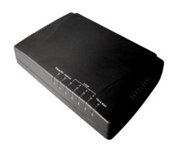
VE1000 is a VDSL to Ethernet Bridge that represents an end-to-end VDSL solution for a 10Mbps Ethernet over a twisted-pair wire. This Ethernet to Phone Line Bridge seamlessly extends your high speed Internet connection, or your existing Ethernet network, to any room in the building or house with a telephone jack. All phone line network products have been designed to operate on the telephone wire installed in homes throughout the world.
